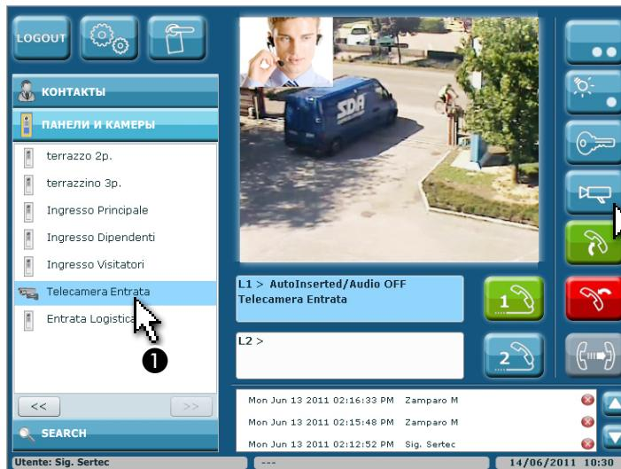
**EN** From the list “Entry panels & Cameras” select any entry panel or camera ① (among the reachable ones); press the key ② to display the images.
